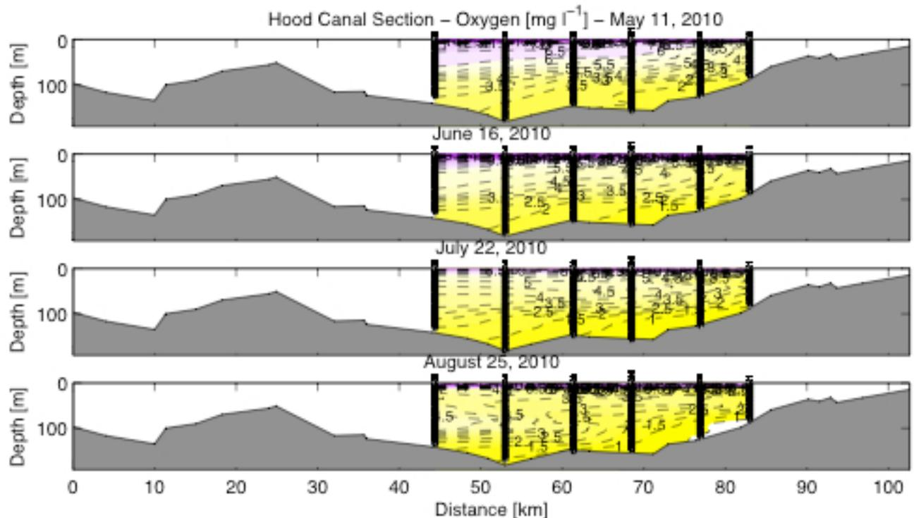
Fig. 5. Sections of oxygen concentration (mg/L) with depth versus horizontal distance between Dabob Bay and the Great Bend for May through August 2010. Data from the HCDOP Citizen Monitoring Program of the HCDOP IAM science study.
