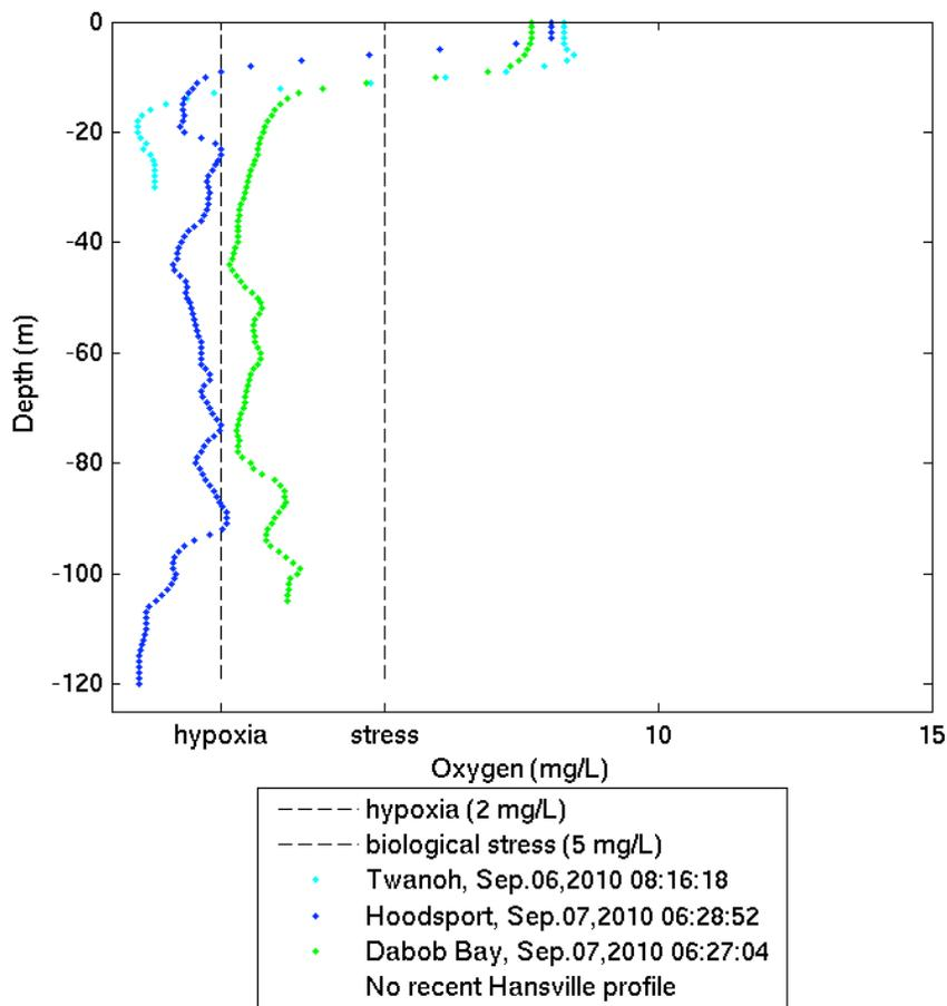
Fig. 3. Latest depth profiles of oxygen from the ORCA buoys in Hood Canal.
