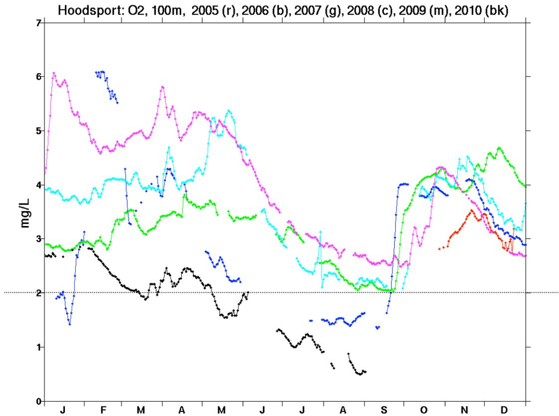
Fig. 2. Oxygen concentration at the HCDOP-NANOOS buoy at Hoodspport in Hood Canal at 100 m depth for 2005 (red), 2006 (blue), 2007 (green), 2008 (cyan), 2009 (magenta), and 2010 (black). Data from the UW ORCA buoy through the HCDOP IAM science study and NANOOS.
